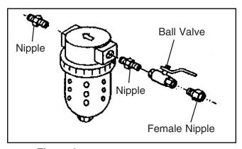
Figure 6. Water separator assembly.
